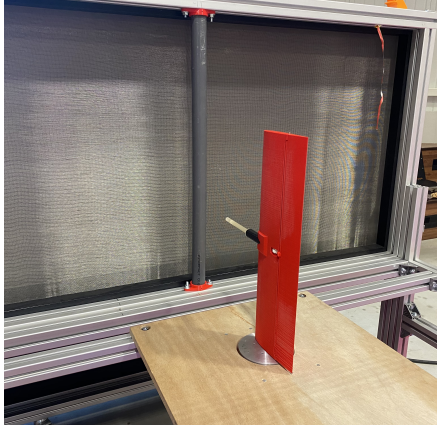
(a) Vortex generator cylinder in front of the WindShape.
