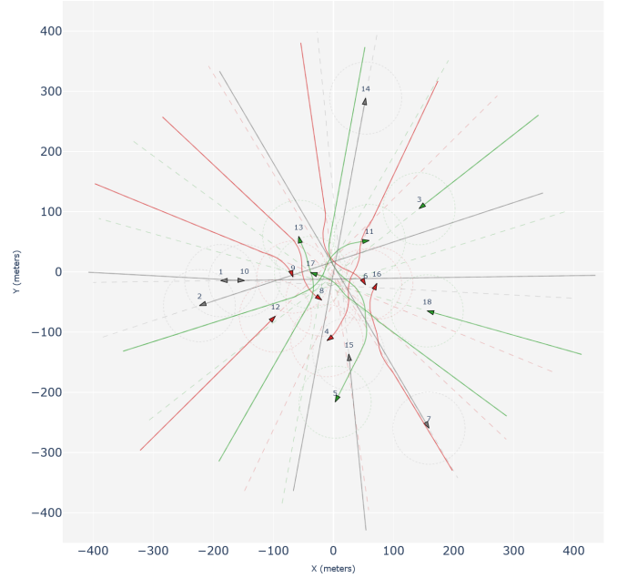
Fig. 1. Multiple deconfliction algorithms, marked with different colored trajectories, operate simultaneously in the same airspace. Dashed lines are the intended flight paths and solid lines are the resultant trajectories after deconfliction efforts. Circles around the vehicles represent the Well-Clear range.
