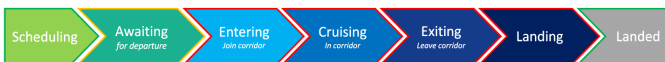
Figure 4. Sequence of operational phases for a single mission, from pre-departure to landing.
